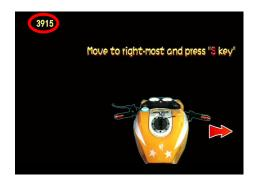
06: Release the throttle and press S key. Reference number range from 200 to 400. Finish correction and automatically back to setup menu. Please save before quit menu.
