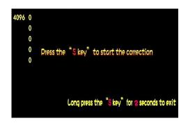
03: Move motorbike to left-most and press S key. **Reference number on range from 4200 to 4400.**
