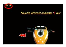
05: Turn the throttle to maximum and hold it then press S key. Reference number range from 700 to 900.
